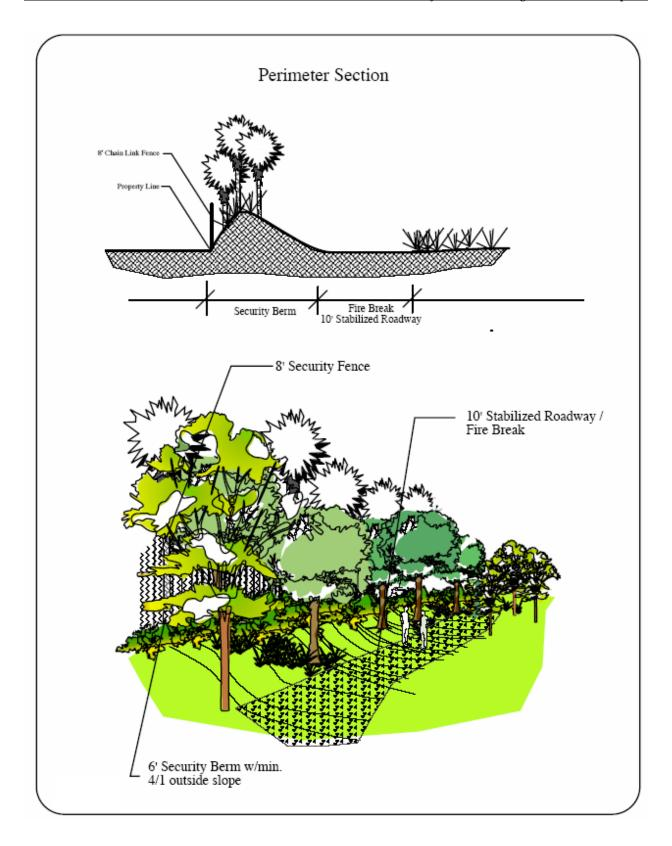
**Figure 8:** Railhead Scrub Preserve Perimeter Fence and Berm
